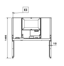
**Electric** Supply voltage: 220-240 V/1 ph/50 Hz Electrical power max: 0.77 kW Capacity: Number and type of grids (included): 6 - GN 2/1 **Key Information:** 1135 lt Net Volume: Door hinges: External dimensions, Width: 1441 mm External dimensions, Depth: 835 mm External dimensions, Depth
